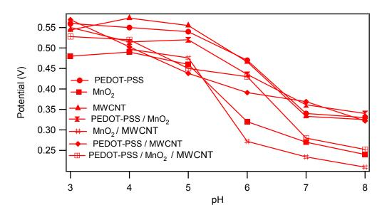
Fig. 3: Peak potentials vs. pH for all modified GCEs
