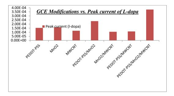
Fig. 1: Different GCE modifications vs. L-dopa peak current
